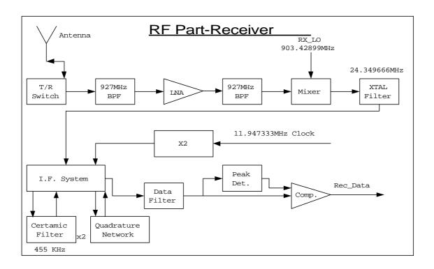
The IF signal enter to crystal filter (BPF) and entered to standard FM discriminator integrated circuit. The output of the discriminator enters to threshold comperator that generates the data signal.
