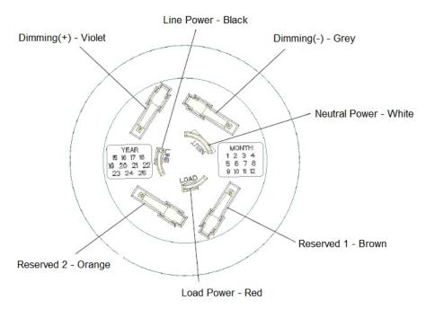
Figure 4 - LCU NEMA 7-Pin Contact Interface
