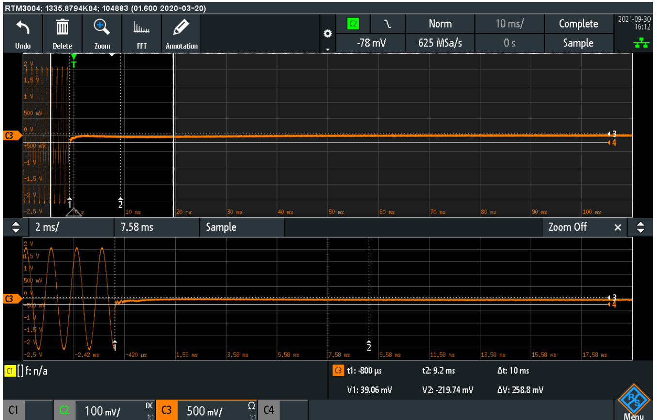
Plot 7.6.7 Transient frequency during power ON test results at high carrier frequency
