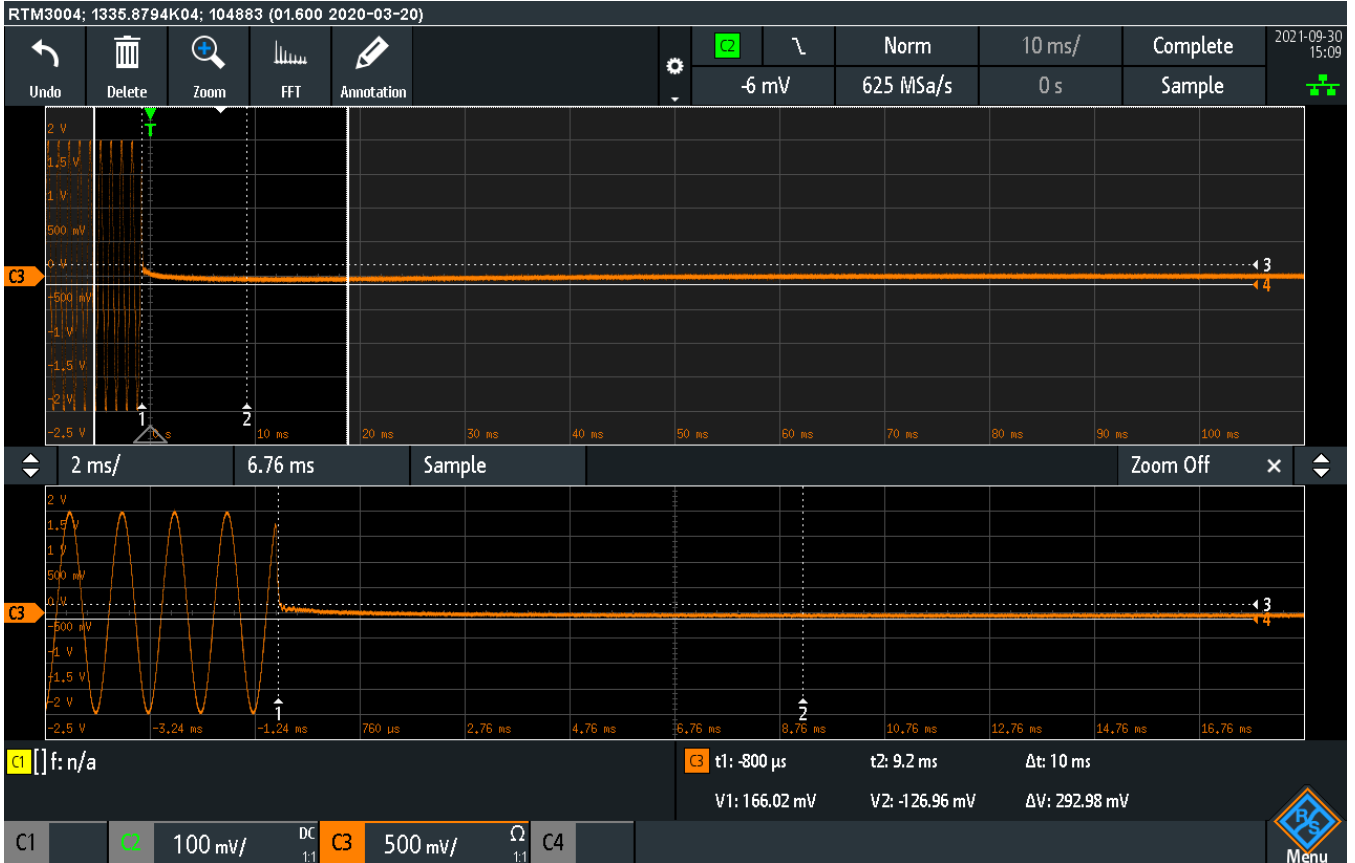
Plot 7.6.1 Transient frequency during power ON test results at low carrier frequency
