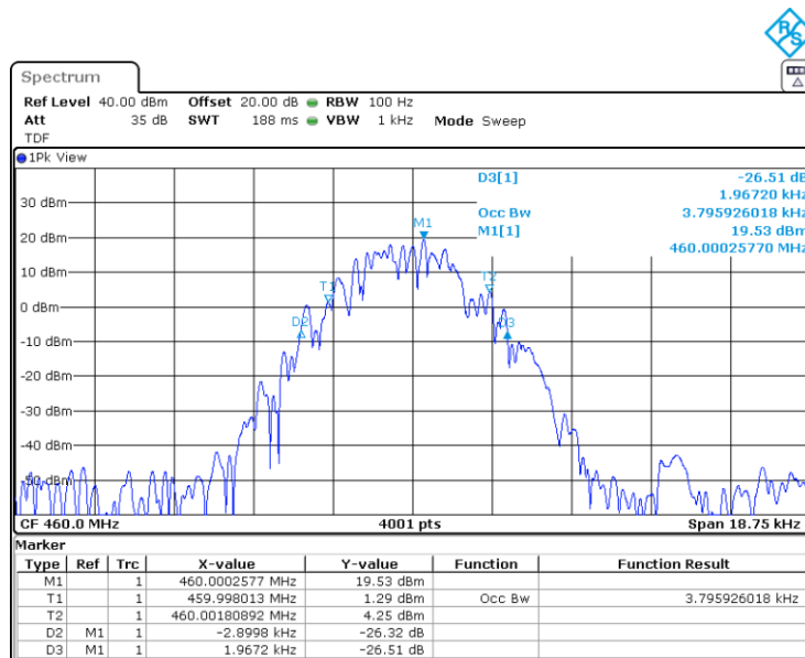
Plot 7.2.2 Occupied bandwidth test result at mid frequency
