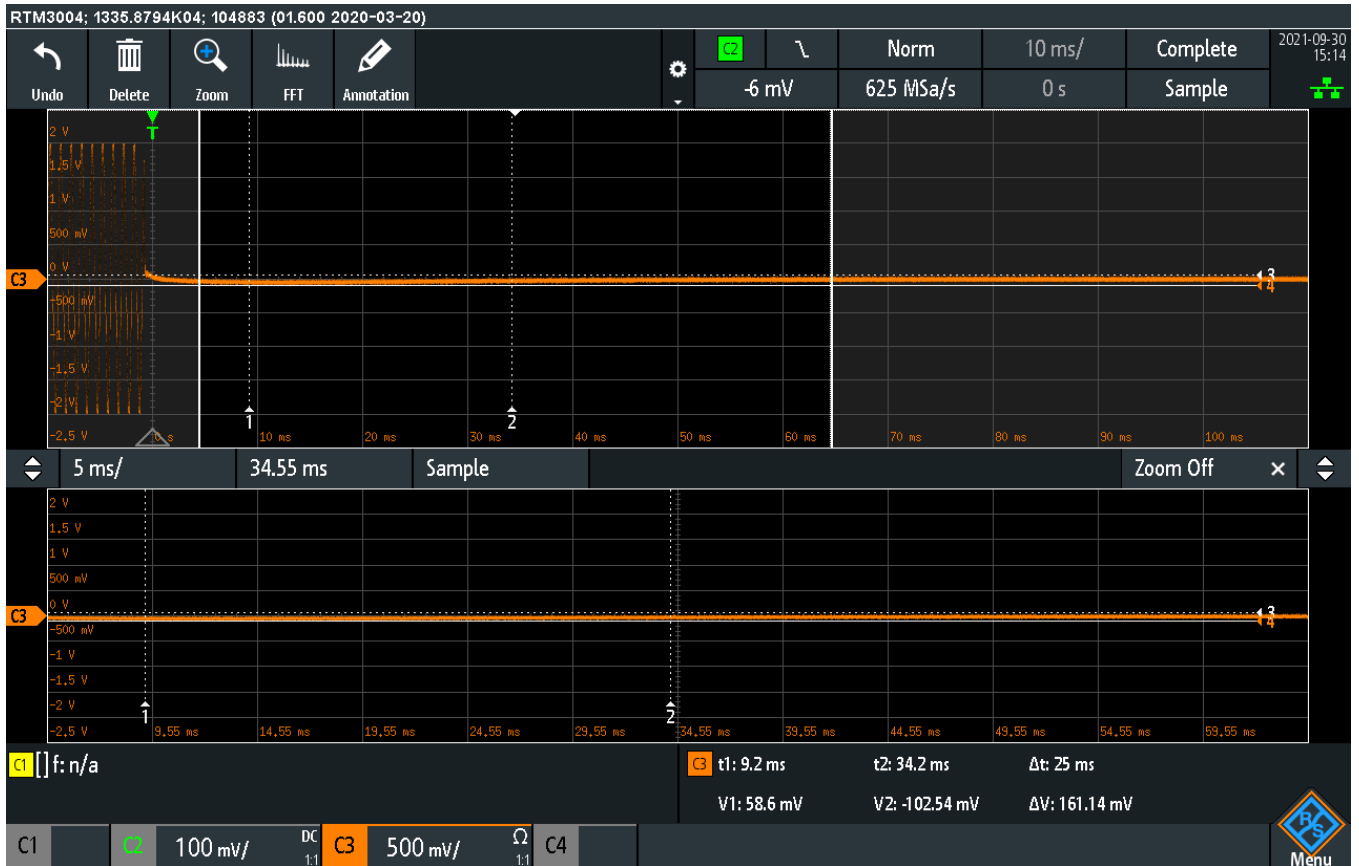
Plot 7.6.2 Transient frequency during power ON test results at low carrier frequency
