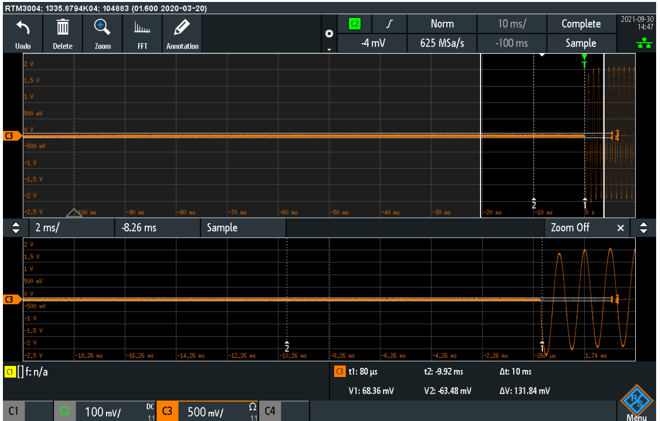
Plot 7.6.3 Transient frequency during power OFF test results at low carrier frequency
