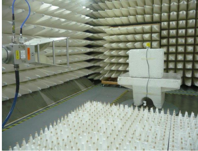
Photograph No.3 Setup for spurious emission field strength measurements in the anechoic chamber above 1000 MHz range
