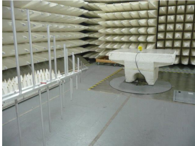
Photograph No.2 Setup for carrier field strength measurements in the anechoic chamber in 30 – 1000 MHz range
