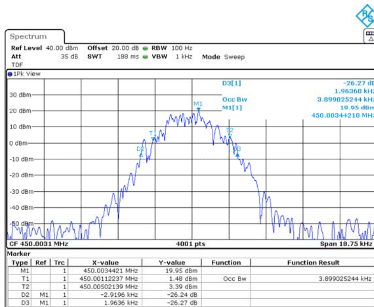
Plot 7.2.1 Occupied bandwidth test result at low frequency
