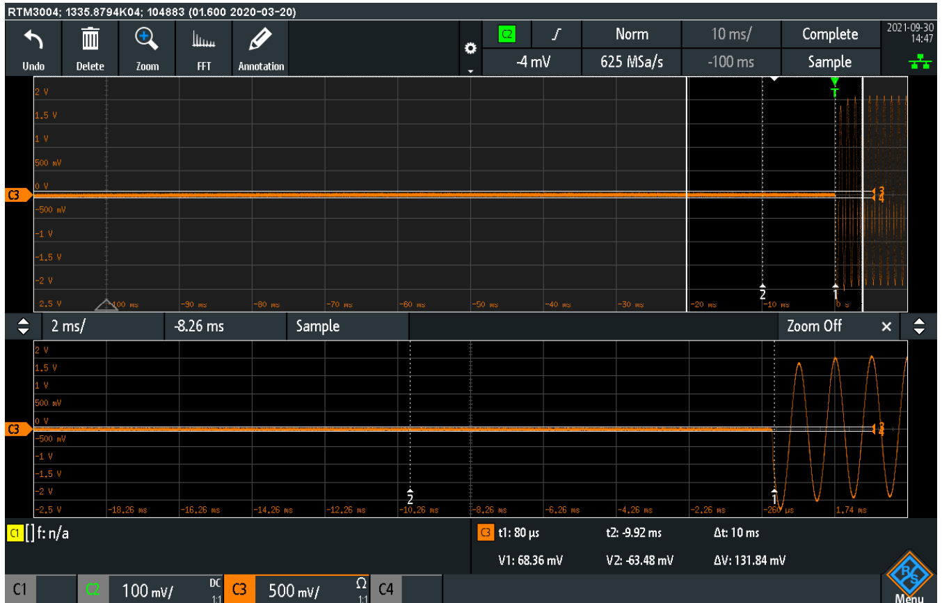
Plot 7.6.6 Transient frequency during power OFF test results at mid carrier frequency
