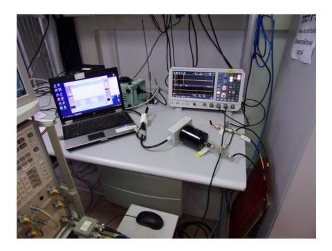
Photograph No.6 Setup for transient frequency behavior measurements
