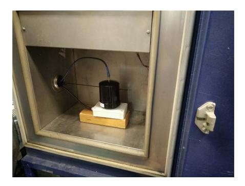
Photograph No.5 Setup for frequency stability measurements
