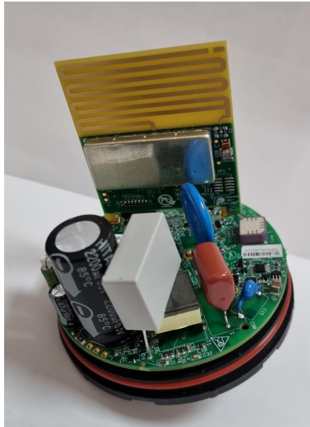
RF and Platform cards assembly
