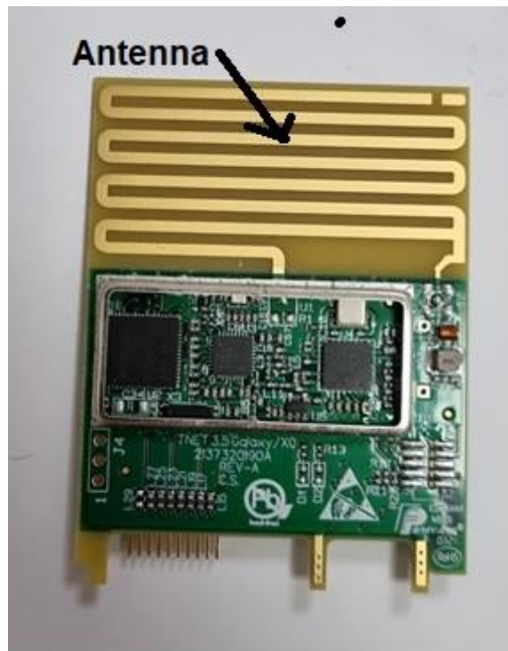
RF Card (TNET3.5) shield removed- top view
