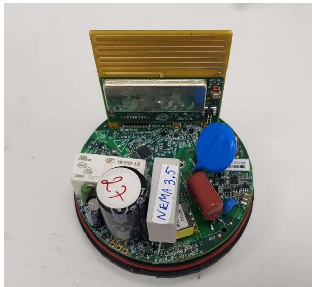
RF and Platform cards assembly
