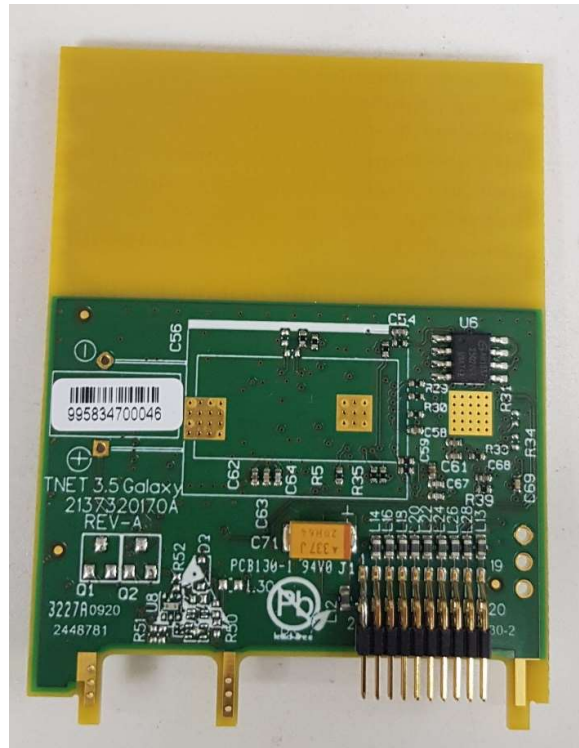
RF Card (TNET3.5) - bottom view
