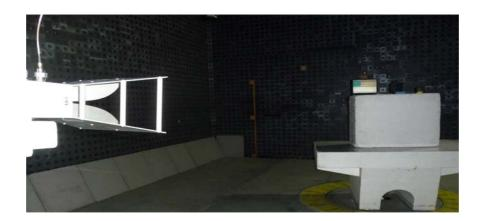
Photograph No.4 Setup for conducted emission measurements on the EUT AC power lines
