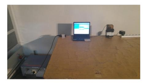
Photograph No.5 Setup for conducted emission measurements on the laptop AC power lines
