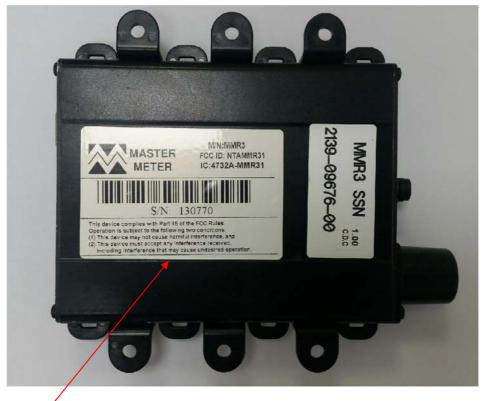
Label with FCC ID:NTAMMR31 and IC:4732A-MMR31 is placed here.
