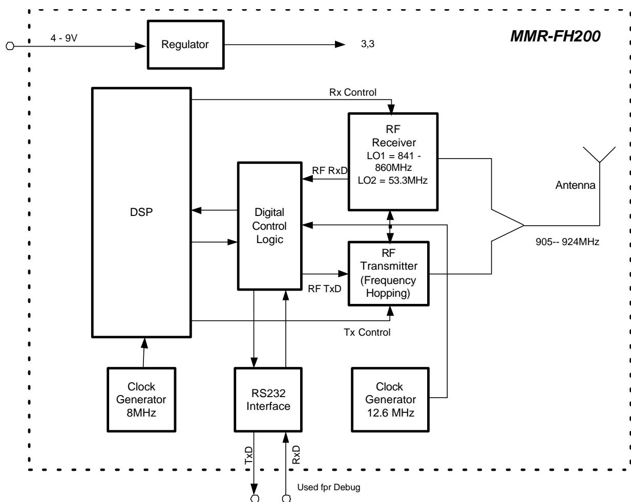
Figure 1: MMR-FH200 Block Diagram
