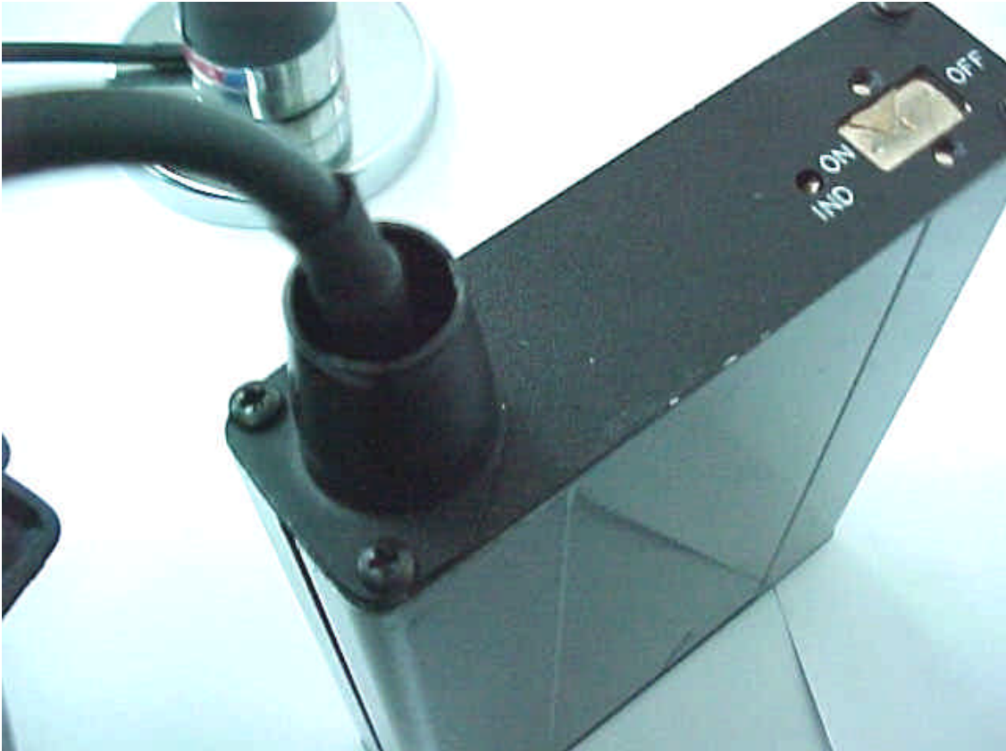
Antenna connector attached to MMR
