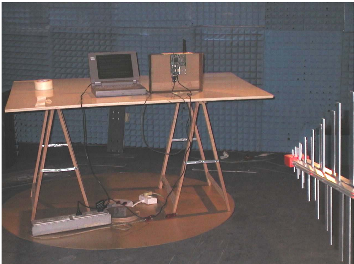
RE/2 Set up for 30MHz-1GHz Portable Configuration with Out Port-Antenna
