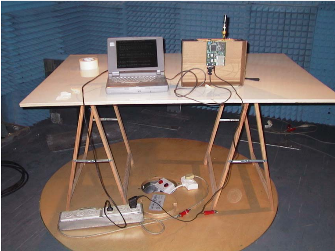
RE/1 Set up for Portable Configuration with Out Port-50ohm
