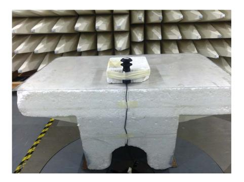
Photograph No.5 Setup for spurious emission measurements in the anechoic chamber above 1000 MHz
