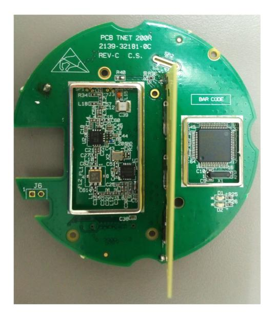
Photograph No.4 LCU RF card top view with shield removed
