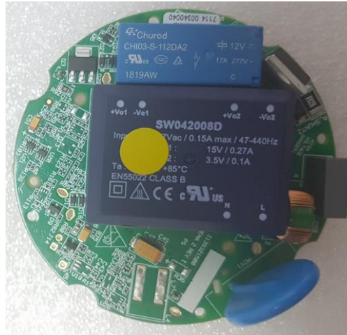
Photograph No.3 Print side of the main PCB
