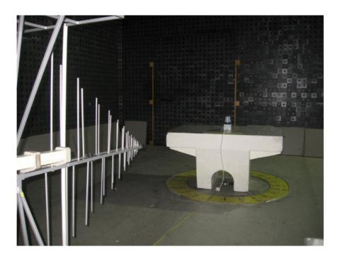
Photograph No.4 Setup for spurious emission measurements in the anechoic chamber above 1000 MHz
