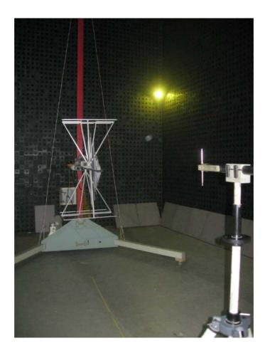
Photograph No.5 Setup for substitution ERP measurements of spurious below 1000 MHz
