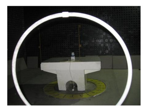
Photograph No.3 Setup for spurious emission measurements in the anechoic chamber below 1000 MHz
