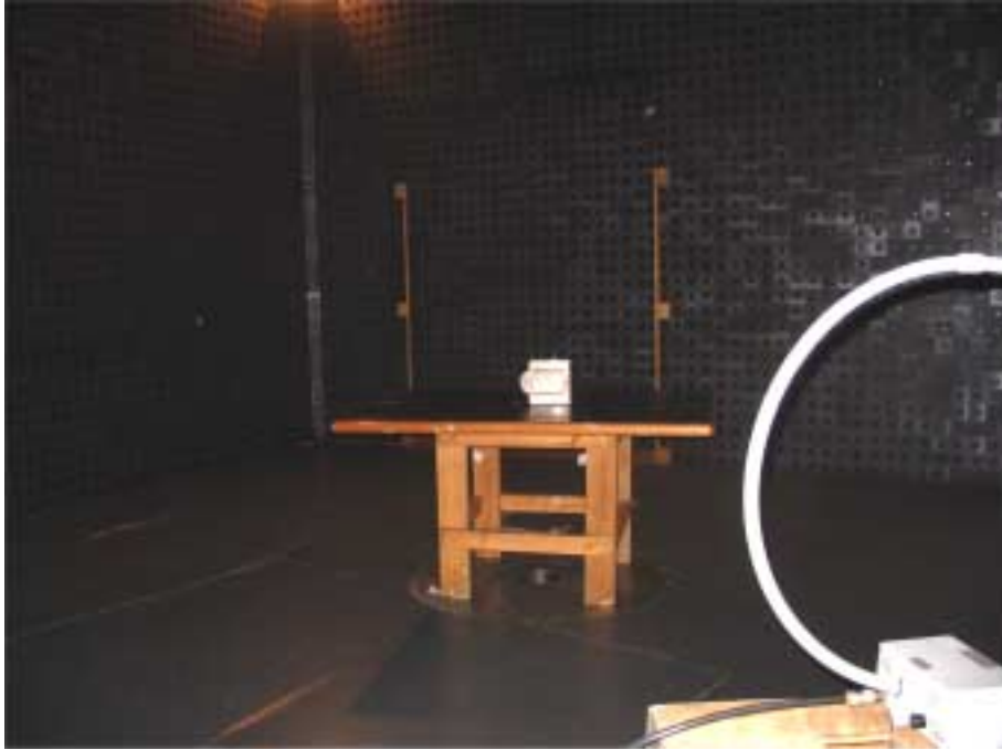
Photograph No.2 Spurious radiated emissions measurement setup in the anechoic chamber with loop antenna
