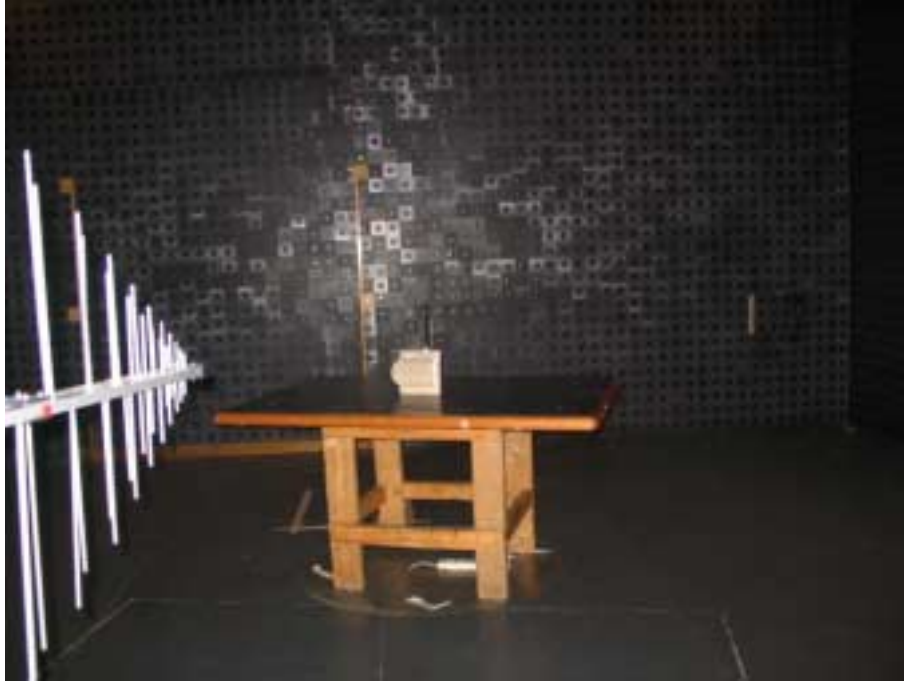
Photograph No.3 Spurious radiated emissions measurement setup in the anechoic chamber with biconilog antenna
