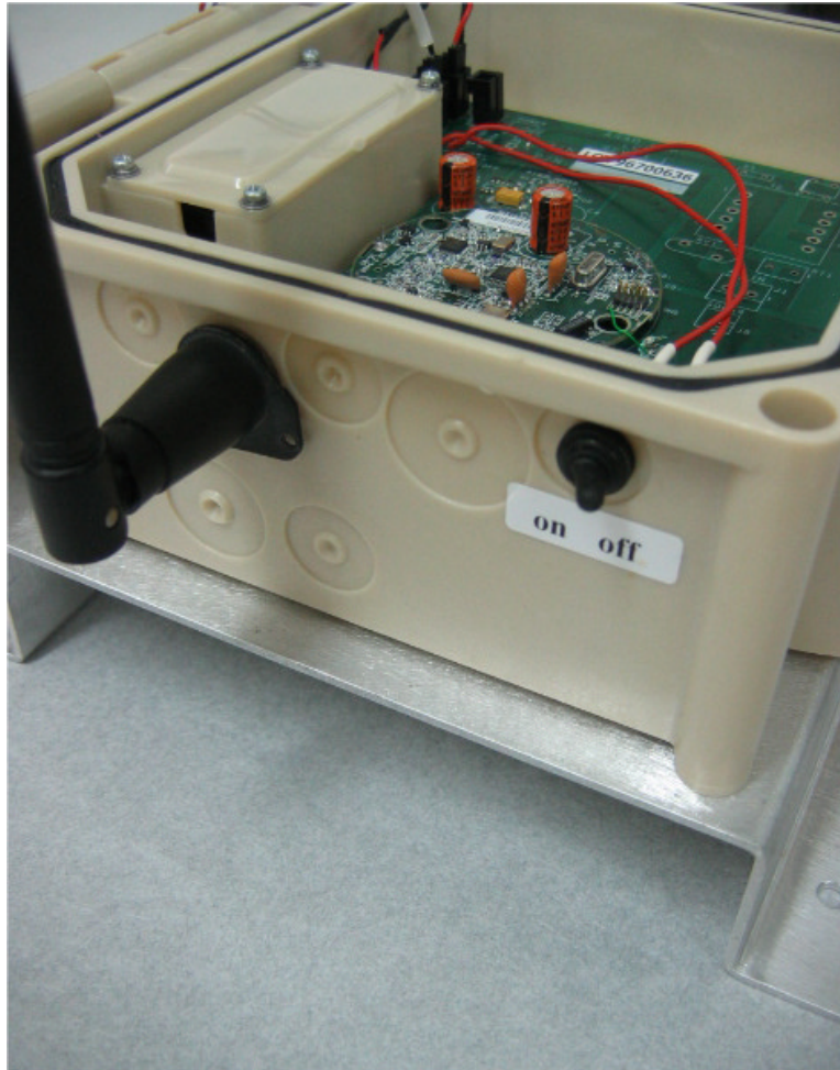
Photograph No.2 Low cost repeater (LCR) Antenna assembly
