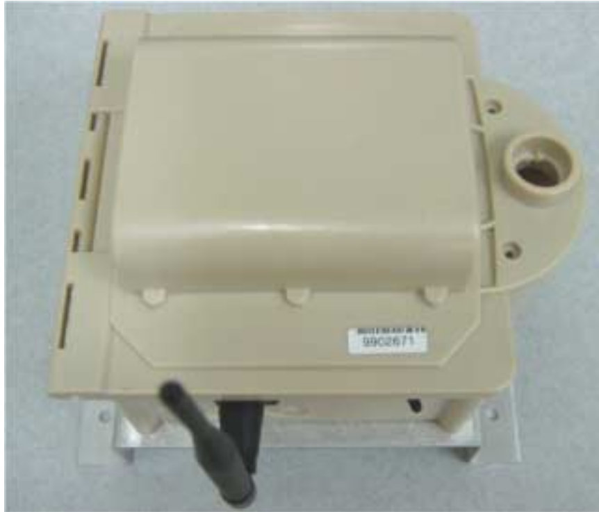
Photograph No.1 LCR (low cost repeater) with antenna Front view
