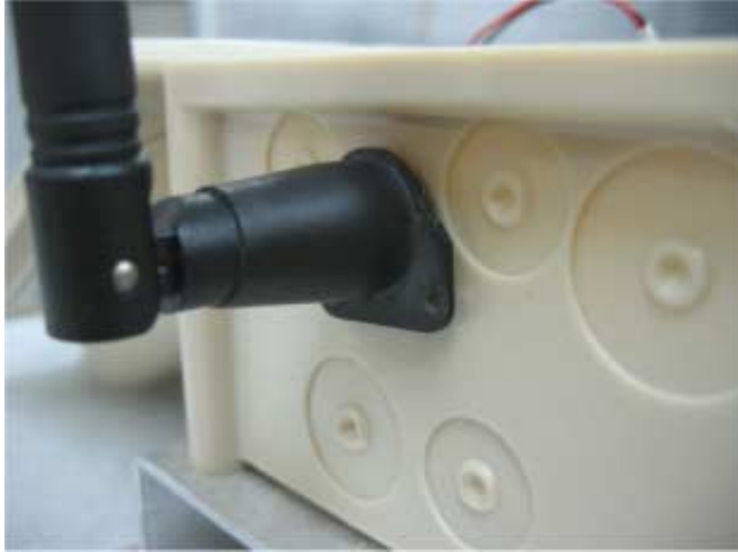
Photograph No.3 LCR antenna connection
