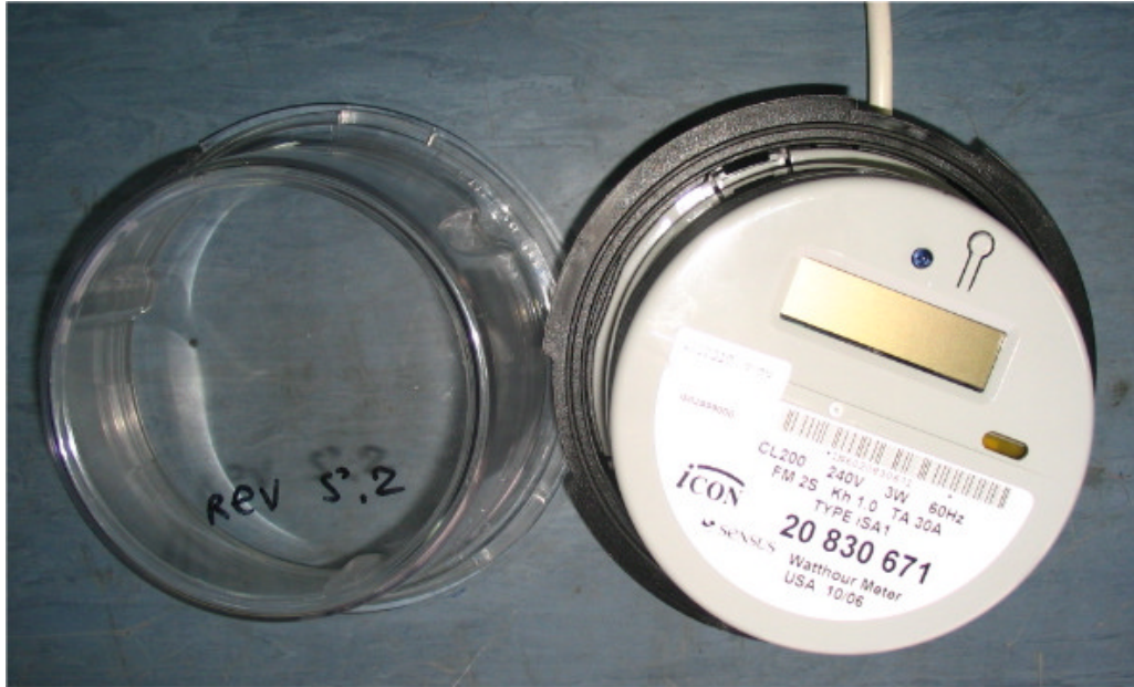
Photograph No.1 ICON240V electricity meter general view with transient cover removed
