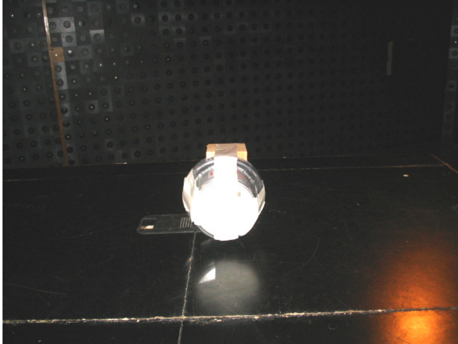
Photograph No.4 Setup for radiated emission measurements in the anechoic chamber, EUT close view
