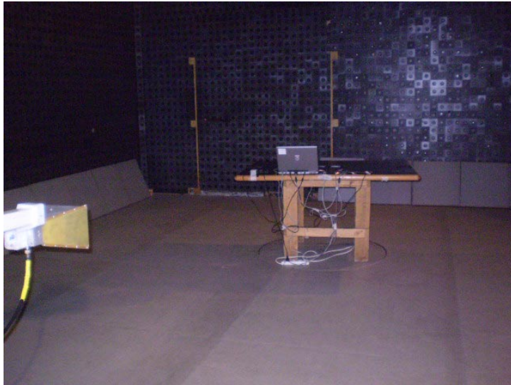
Photograph 7.2.3 Setup for radiated emission measurements, EUT cabling
