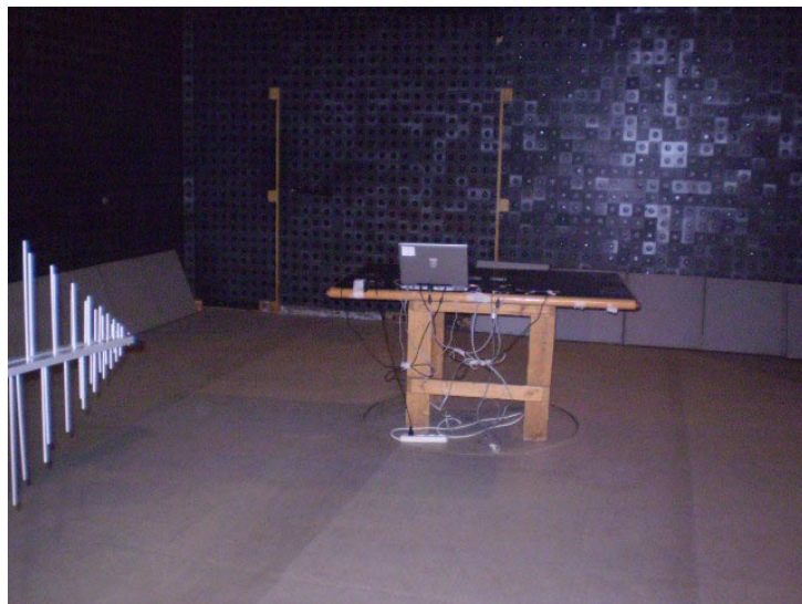
Photograph 7.2.1 Setup for radiated emission measurements in 30-1000 MHz
