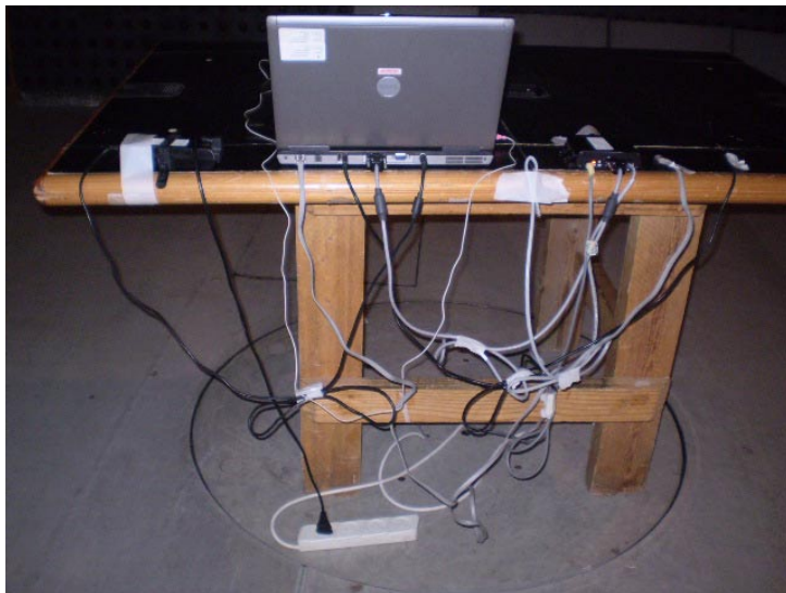
Photograph 7.2.3 Setup for radiated emission measurements, EUT cabling
