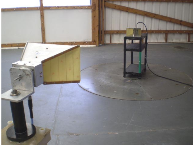
Photograph No.7 Setup for substitution ERP measurements of spurious at the OATS above 1000 MHz
