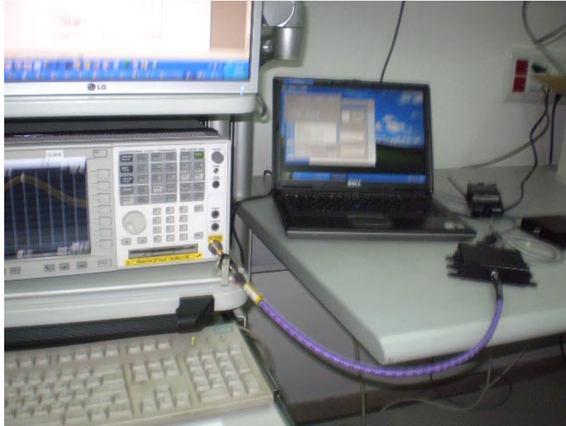
Photograph No.1 Setup for output power, occupied bandwidth, emission mask and conducted spurious emission measurements
