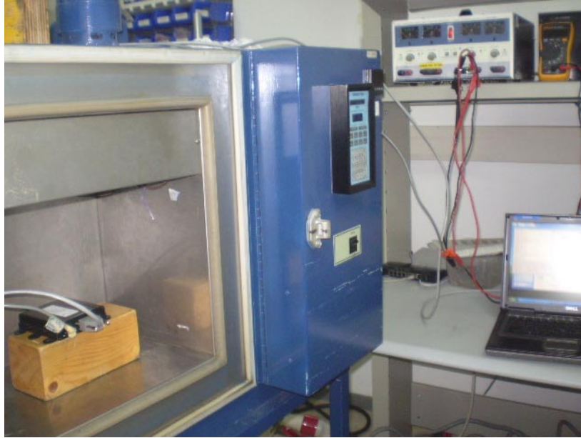
Photograph No.8 Setup for frequency stability measurements
