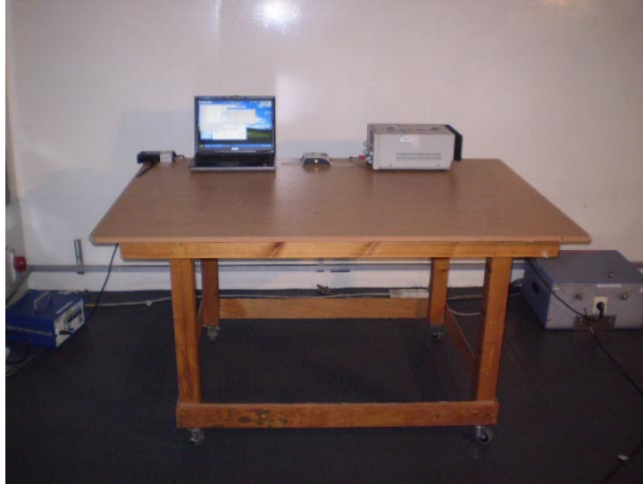
Photograph No.9 Setup for conducted emission measurements on the power lines
