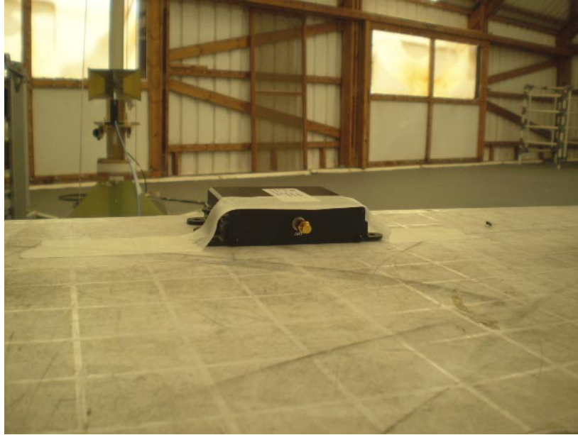
Photograph No.6 Setup for spurious emission measurements at the OATS above 1000 MHz, EUT close view
