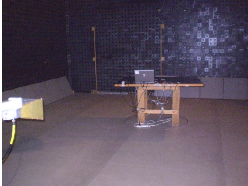
Photograph No.4 Setup for radiated emission measurements in the anechoic chamber above 1000 MHz
