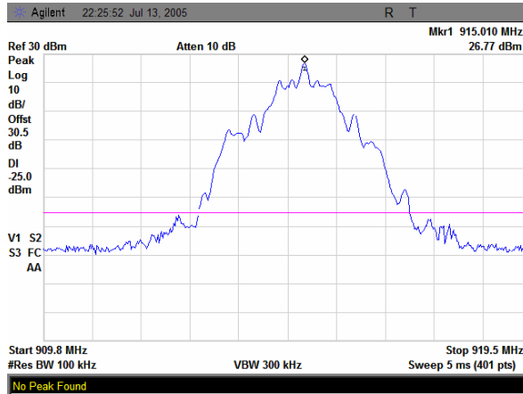
Plot 7.4.24 Spurious emission measurements in 909.8 – 922.5 MHz range at high carrier frequency
