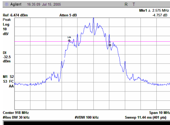
Plot 7.2.3 Occupied bandwidth test result at high carrier frequency
