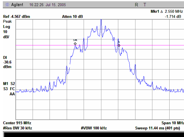
Plot 7.2.3 Occupied bandwidth test result at high carrier frequency
