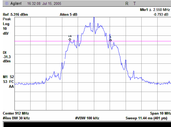
Plot 7.2.2 Occupied bandwidth test result at mid carrier frequency
