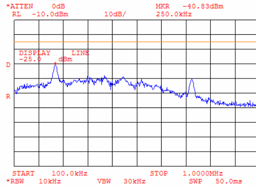
Plot 7.4.6 Spurious emission measurements in 0.10 - 1.0 MHz range at high carrier frequency
