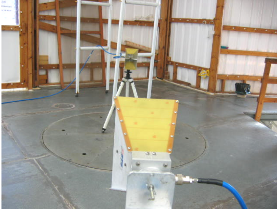
Photograph No.2 Substitution method of power density measurement setup
