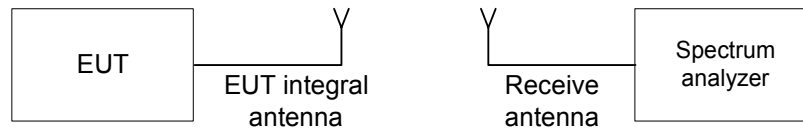
Figure 8.3.1 Emission mask test setup
