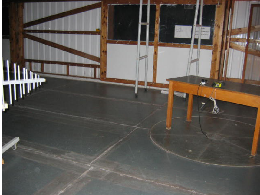
Photograph No.9 Setup for carrier field strength measurements (according to FCC Part 90)
