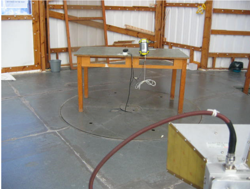
Photograph No.1 Output power, field strength and the 6 dB occupied bandwidth measurement setup
