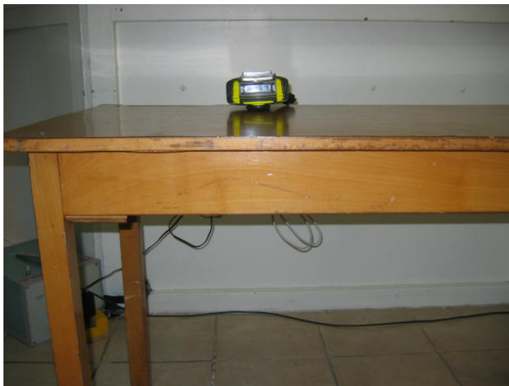
Photograph No.8 Conducted emissions measurement setup
