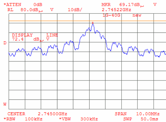
Plot 7.4.11 Radiated emission measurements at the 4 th harmonic
