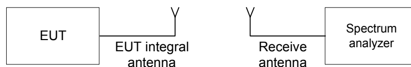
Figure 7.3.1 Emission mask test setup
