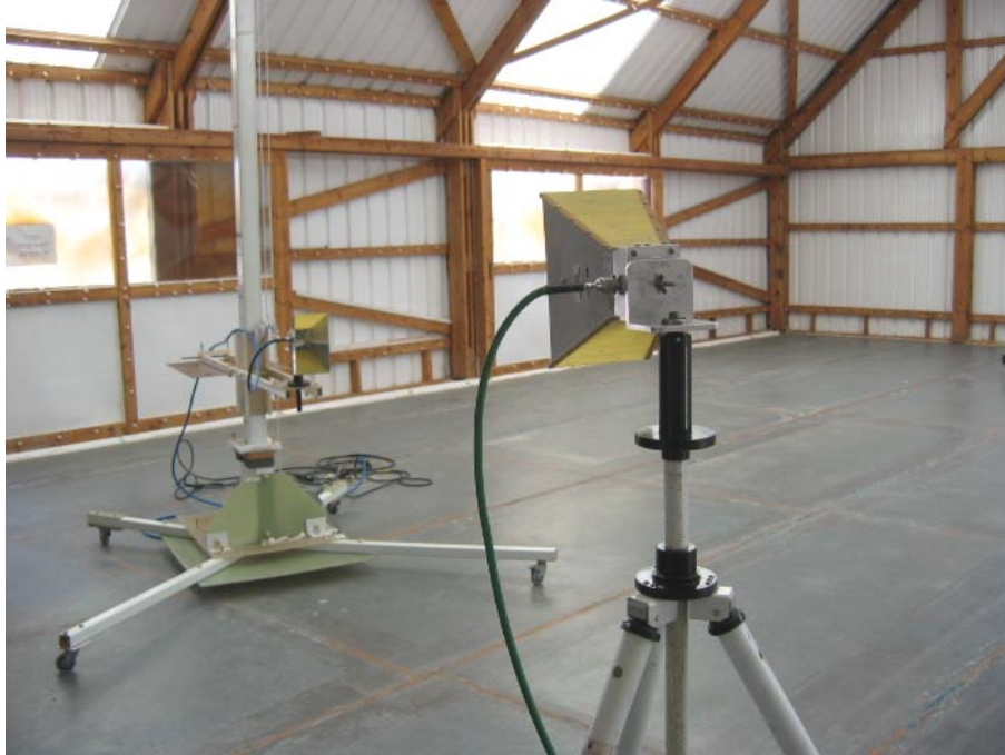
Photograph No.5 Setup for substitution ERP measurements of spurious at the OATS above 1000 MHz
