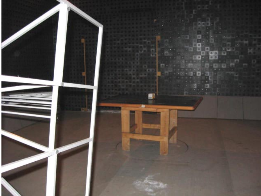
Photograph No.4 Setup for radiated emission measurements in the anechoic chamber from 30 to 1000 MHz
