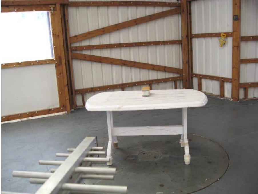
Photograph No.1 Setup for carrier field strength and spurious measurements at the OATS
