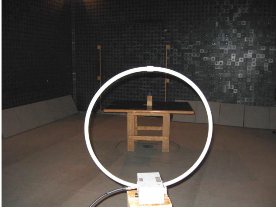
Photograph No.3 Setup for spurious emission measurements in the anechoic chamber below 30 MHz
