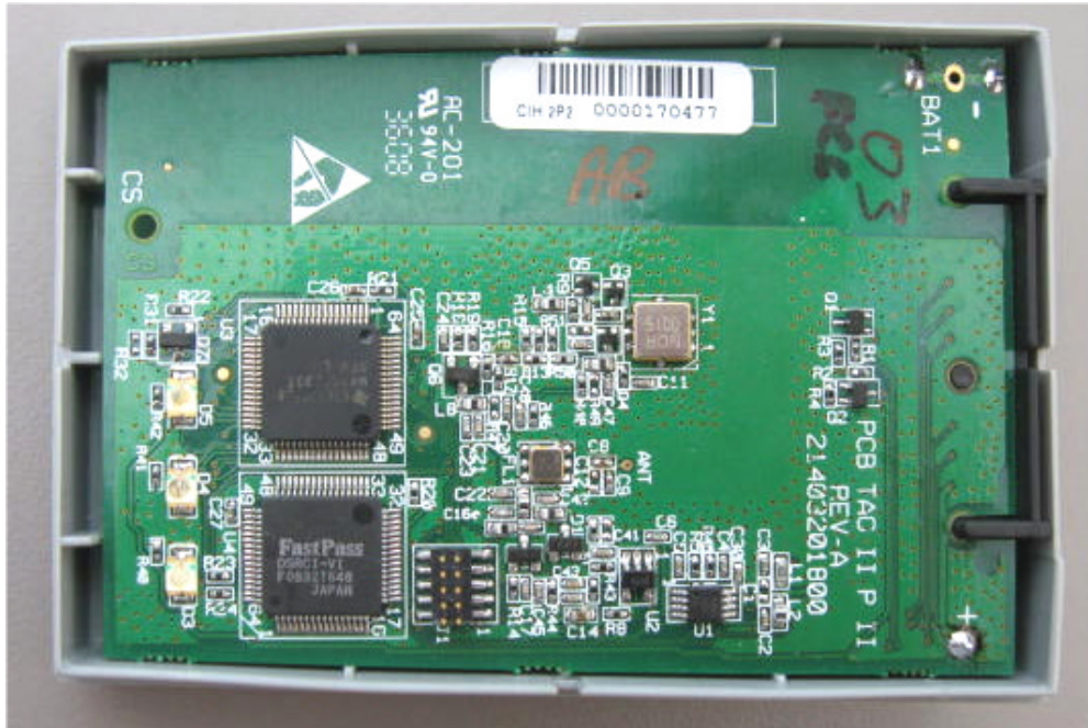
Photograph No.2 Mobile transponder FP101TB internal view without cover
