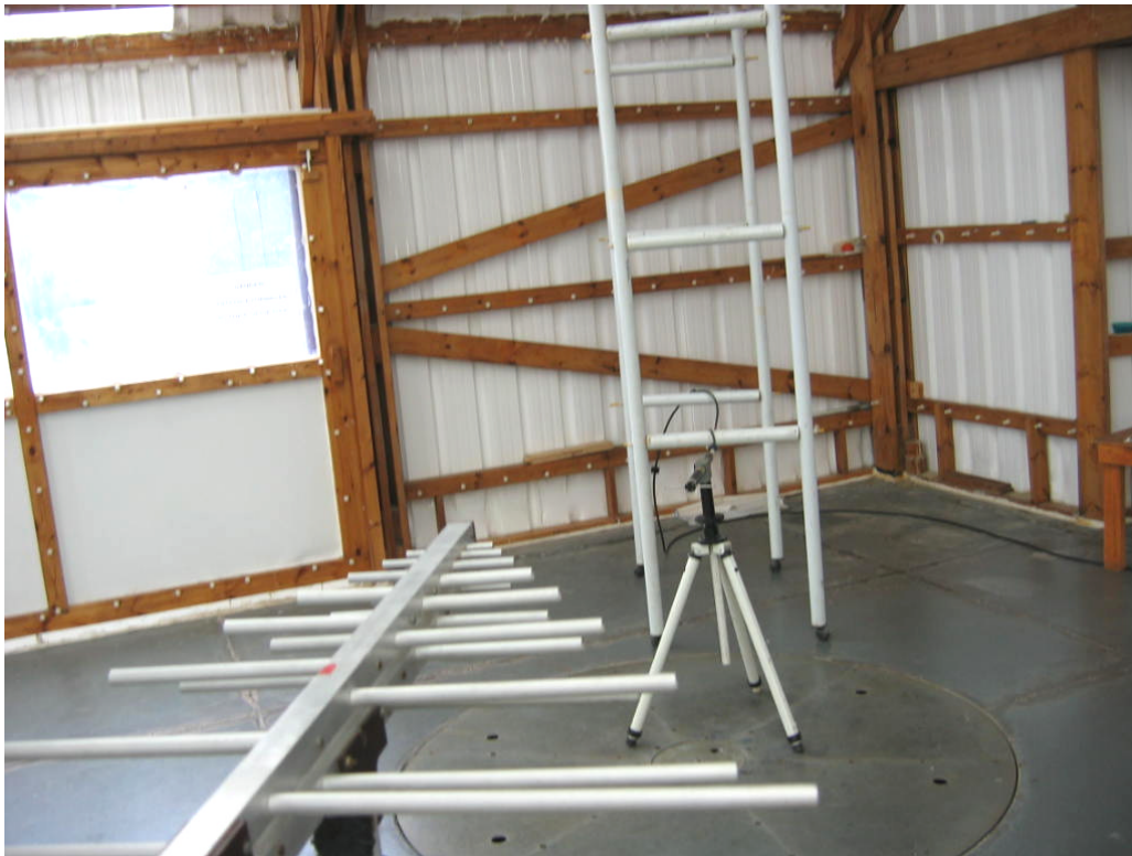
Photograph No.2 Substitution method measurement setup
