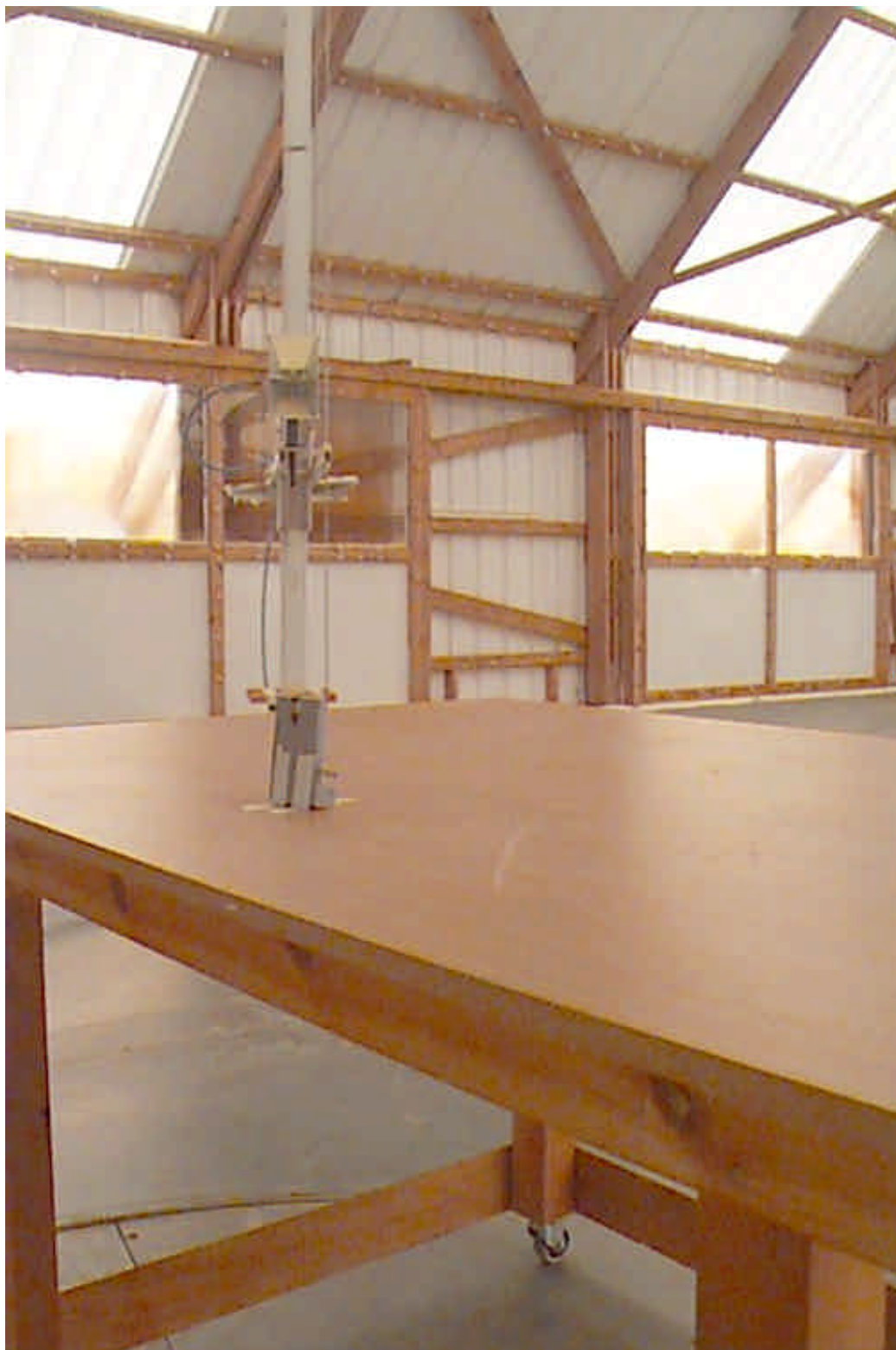
Photograph No.4 Radiated emissions measurement setup at the OATS with double ridged guide antenna
