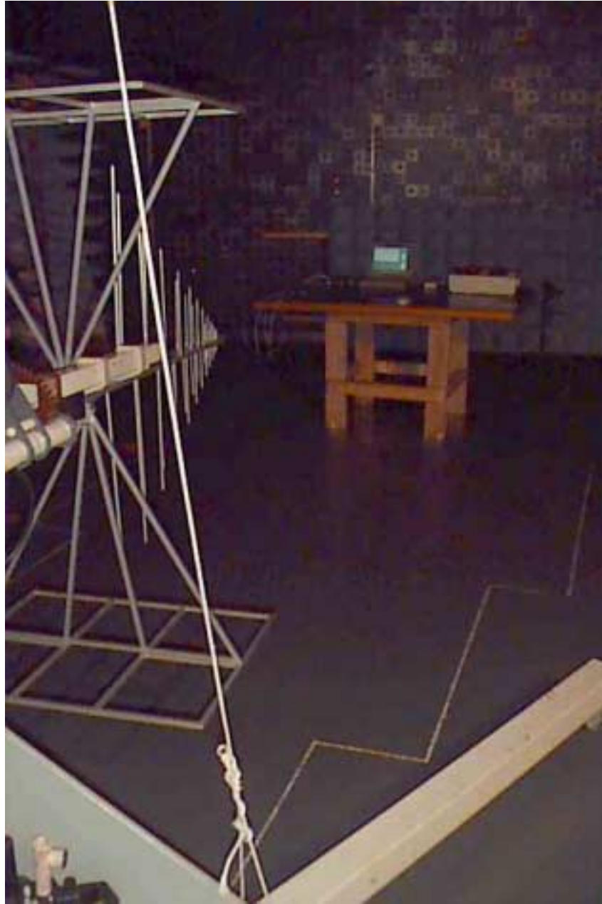
Photograph No.5 Unintentional radiated emissions measurement setup in the anechoic chamber with biconilog antenna
