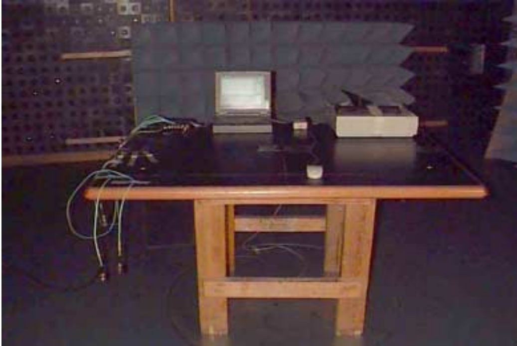
Photograph No.7 Unintentional radiated emissions measurement setup in the anechoic chamber close view
