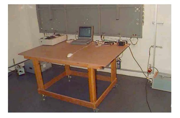
Photograph No.1 Conducted emissions measurement setup
