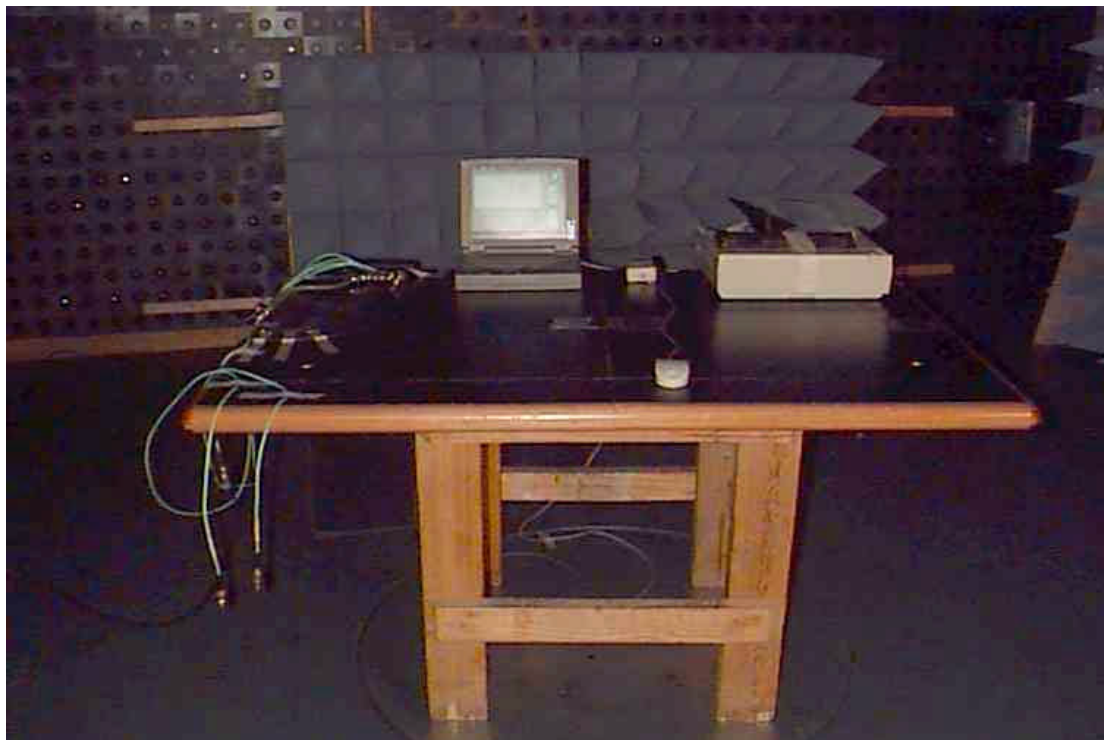
Photograph No.3 Unintentional radiated emissions measurement setup in the anechoic chamber close view
