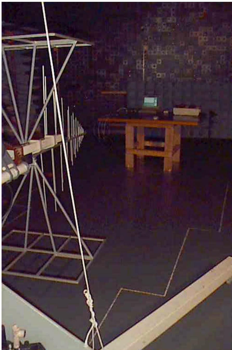
Photograph No.1 Unintentional radiated emissions measurement setup in the anechoic chamber with biconilog antenna
