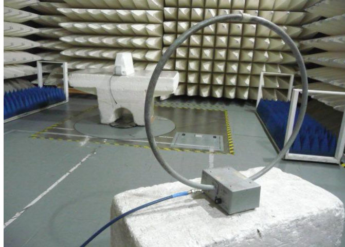
Photograph No.1 Setup for spurious emission field strength measurements in the anechoic chamber below 30 MHz
