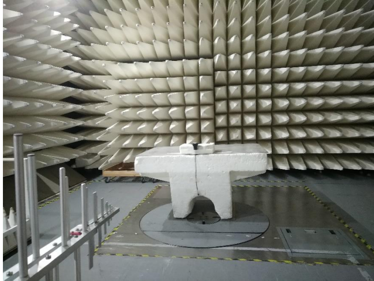
Photograph No.3 Setup for spurious emission measurements in the anechoic chamber above 30 MHz
