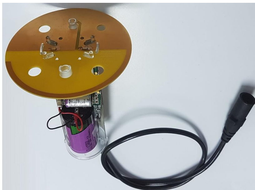
Antenna- Top Assembly
