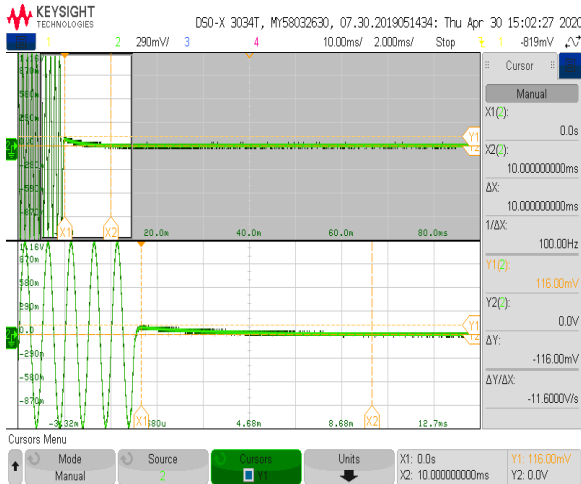
Plot 7.6.5 Transient frequency during power ON test results at high carrier frequency
