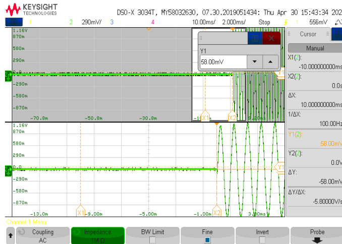
Plot 7.6.6 Transient frequency during power OFF test results at high carrier frequency
