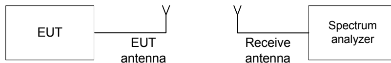
Figure 7.7.1 Band edge emission test setup
