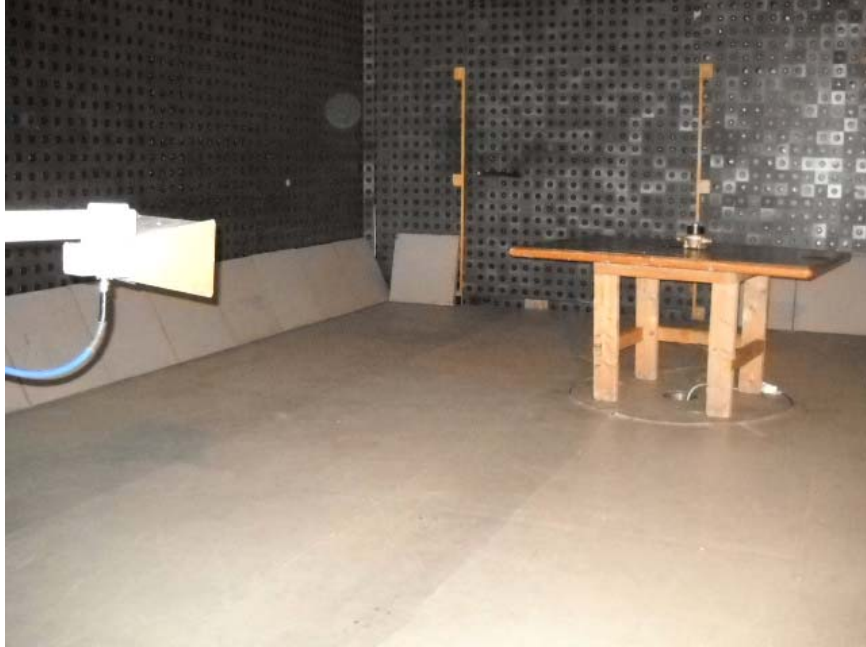
Photograph No.3 Setup for spurious emission measurements in the anechoic chamber above 1000 MHz
