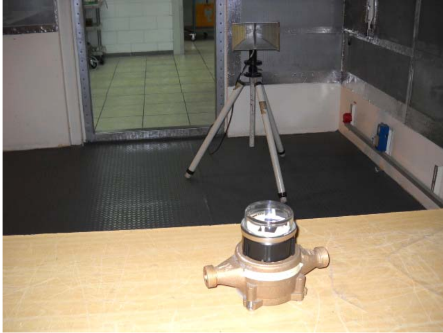
Photograph No.4 Hopping parameters measurement test setup
