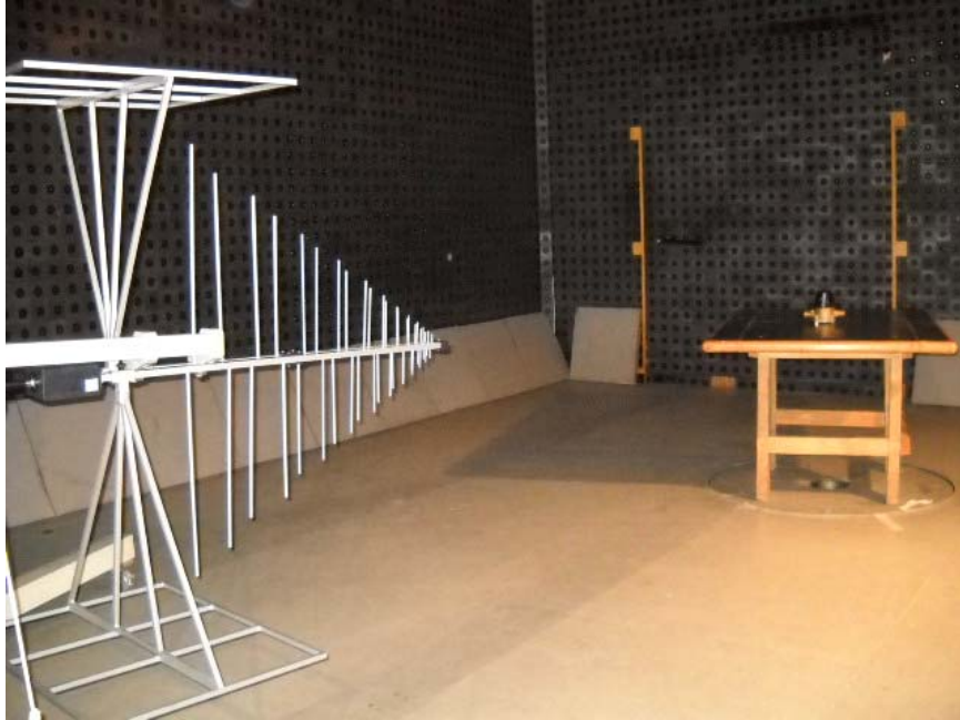
Photograph No.1 Setup for carrier power, spurious emissions field strength and 6 dB OBW measurements in the anechoic chamber from 30 to 1000 MHz
