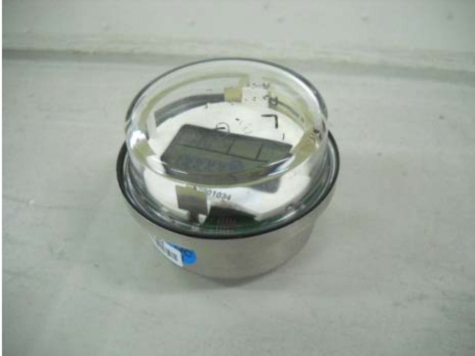
Photograph No.1 “3G interpreter LG” water meter extracted from external enclosure
