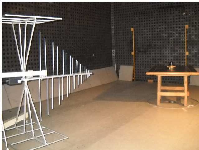
Photograph 8.1.1 Setup for radiated emission measurements, general view
