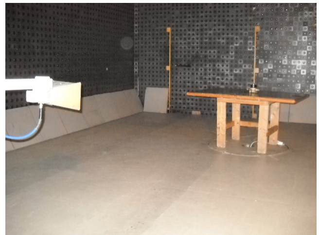
Photograph 8.1.1 Setup for radiated emission measurements, general view
