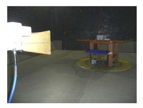
Photograph No.5 Setup for spurious emission measurements in the anechoic chamber, EUT close view
