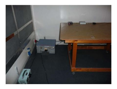
Photograph No.9 Conducted emission on AC power lines test setup
