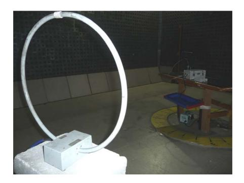
Photograph No.3 Setup for spurious emissions measurements in the anechoic chamber from 30 to 1000 MHz
