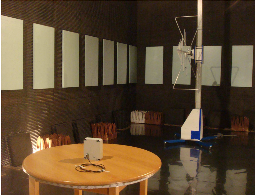
Figure 2.5.1 Radiated measurements below 1 GHz
