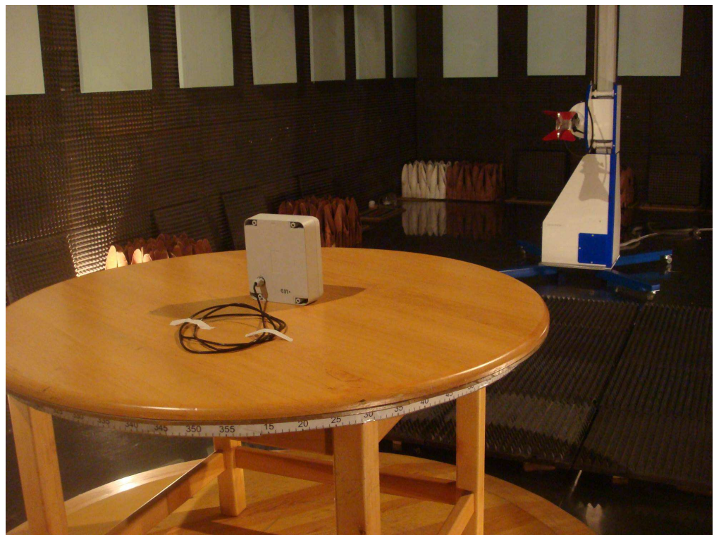
Figure 2.5.2 Radiated measurements above 1 GHz
