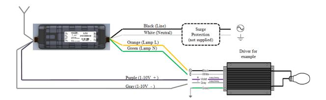
The wiring color for the AC IN/OUT wires:
