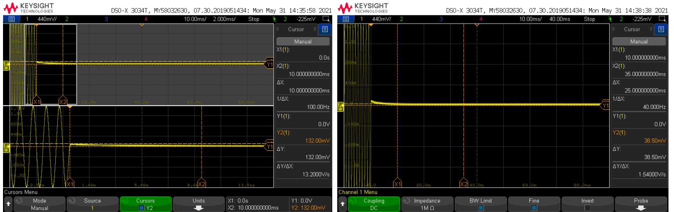
Plot 7.7.3 Transient frequency during power ON test results at mid carrier frequency
