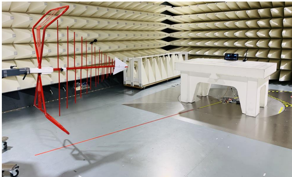
Figure B4: Radiated Emission testing low range Setup
