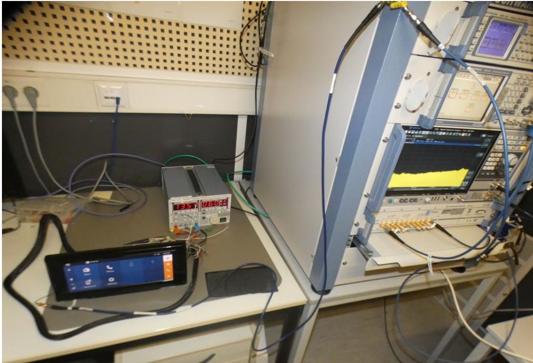
Photo 5: Test setup for conducted measurements
