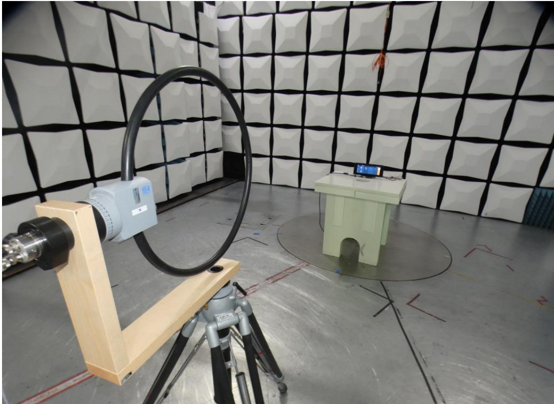
Photo 1: Test setup for radiated measurements (9 kHz - 30 MHz)
