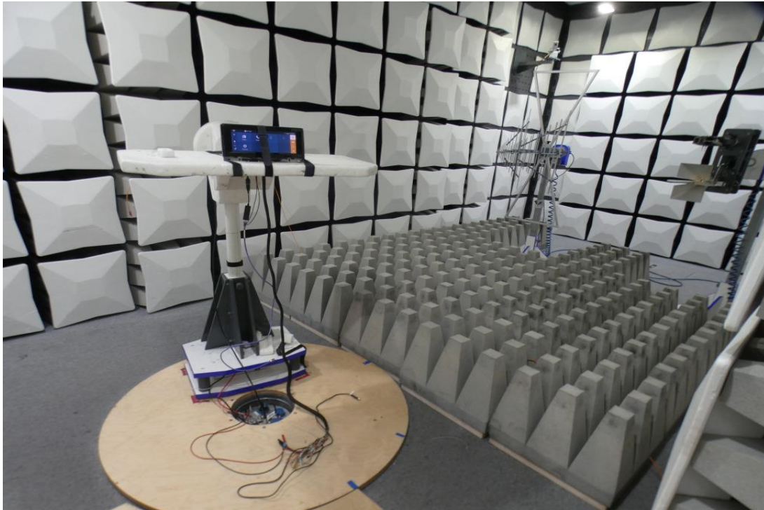
Photo 3: Test setup for radiated measurements (1 GHz – 26 GHz)
